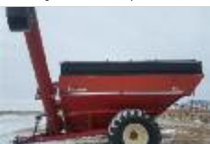
Grain Cart Parker 938 (2011), 950 minots, vis 17", balance, toile, clapet hydraulique, pneu 900/60-32
